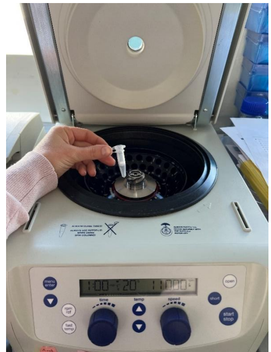
Fig. 8: Purification of the plasmid DNA in a silica membrane column (when put into a centrifuge)
