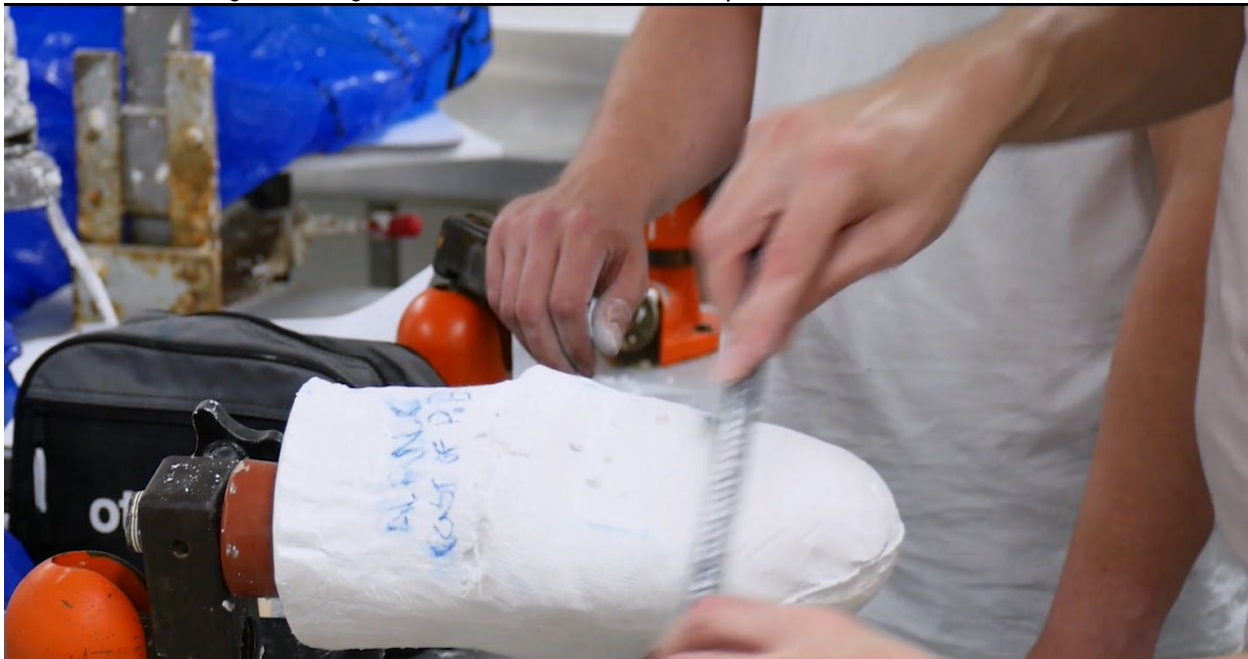
Picture 8: Traditional Stump mold being polished for examining the optimal socket fit. 23
