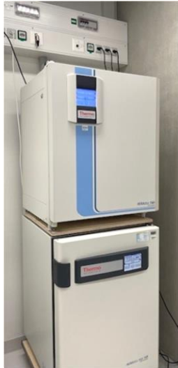
Fig. 5 Incubator used for the controlled growing of cell systems at the Biozentrum Basel
