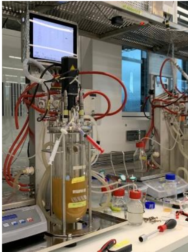
Figure 4 Culturing E. coli by fermentation
