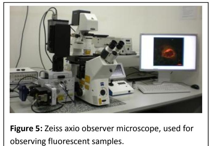
**Figure 5:** Zeiss axio observer microscope, used for observing fluorescent samples.
