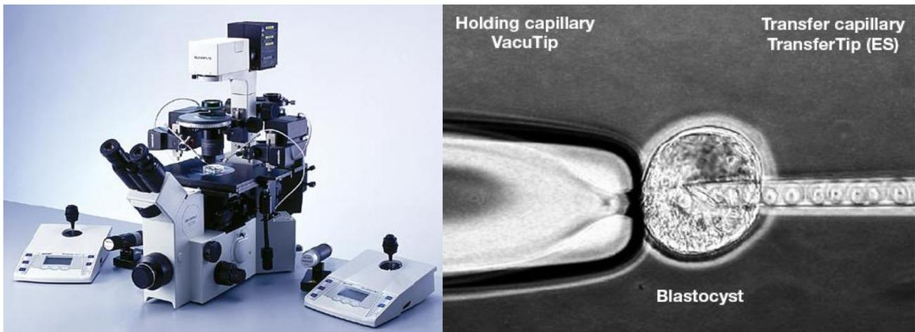
**Figure 6:** Equipment used in embryonic stem cell transfer into a blastocyst (because of the minute sizes, the process is highly mechanized). Shown here are: TransferMan NK2, CellTram Air, CellTram vario and an Olympus IX 70 microscope. On the right is a picture of the actual transfer.
