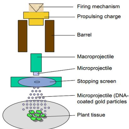
Fig. 5: biolistic transformation, schematical
