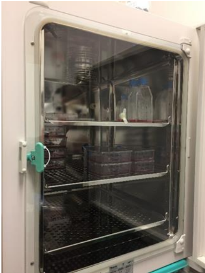
Figure 6. An incubator. It is used to give cell cultures the ideal temperatures to grow.
