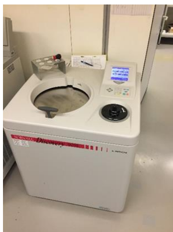
Figure 8. Ultra centrifuge. Centrifuges are used to separate samples into their different components.
