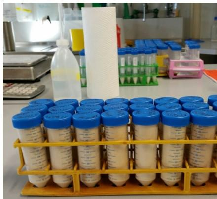
Figure 8: Sample material after grinding, filled into sample tubes; in the background: tubes for weighing the sample quantity for DNA extraction from the ground sample
