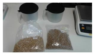
Figure 7: Samples in the laboratory before grinding: 1) soybeans (left) and 2) soycake as feed, pelleted (right); in the background grinding bowl and balance
