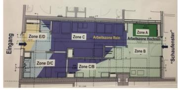
Figure 8 Clean Room Arrangement at the University of Basel
