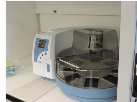
Fig. 2 A machine used in the magnetic beads technique to "fish" out the beads
