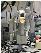
Figure 7: 12-channel adjustable volume pipettes. Such pipettes are used to generate multiple same (pro)portions of a solution. This is a faster way preparing substances.
