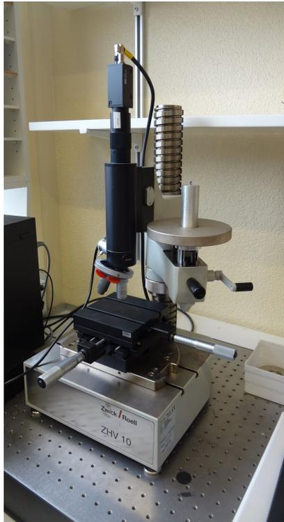
Fig.3: Light microscope with camera on the left arm and Diamond Tip with crank on the right arm. (AELEN, 2018)
