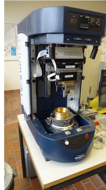
Fig. 4: Picture of an opened and inactive tribometer. (AELEN, 2018)
