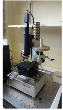
Another measuring apparatus is the one in figure 3. It's a diamond tip which is pressed into the material to then visually observe repression with the light microscope which is on the second arm of it.
